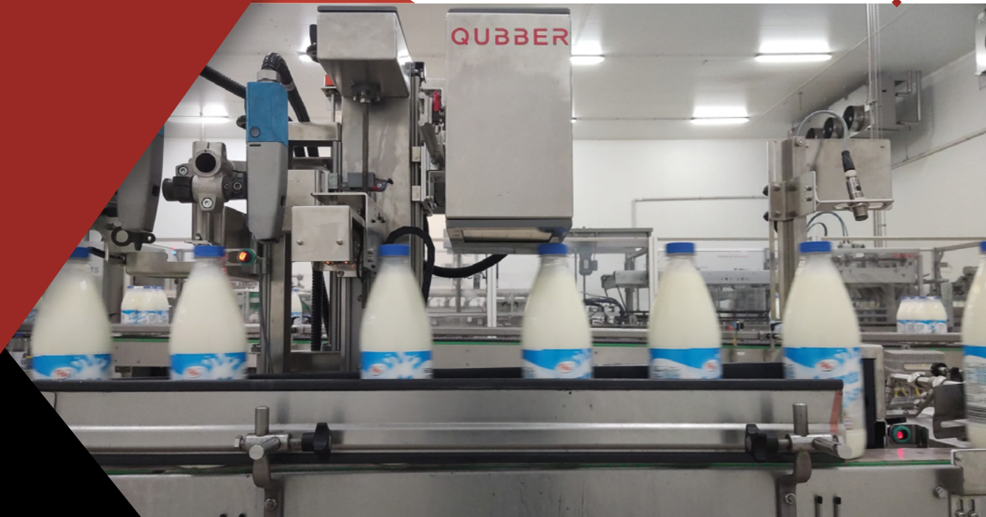
Module for expiration date inspection
